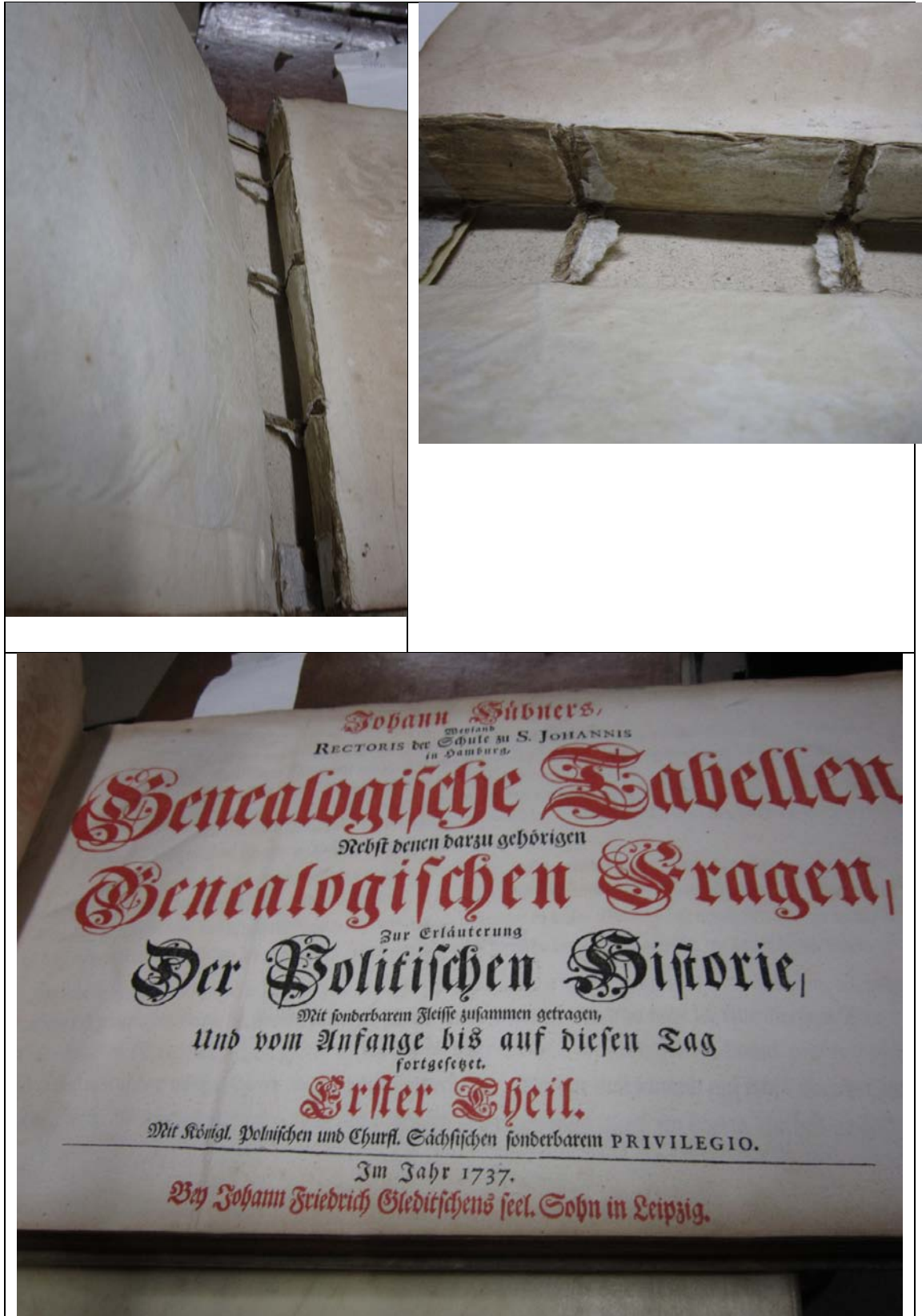
Head cut too short. Cords cut in and glued, not sewn.
